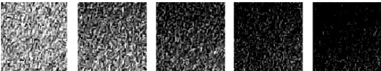
Fig. 3 - Amplitude spectra of surface images of St3 steel samples in the range of gray scale gradations at different stages of fatigue in the range of relative durability under gigacycle loading: a - 10^6 ; b - 10^7 ; c - 10^8 ; d - 10^9 ; e - 10^{10} cyc
